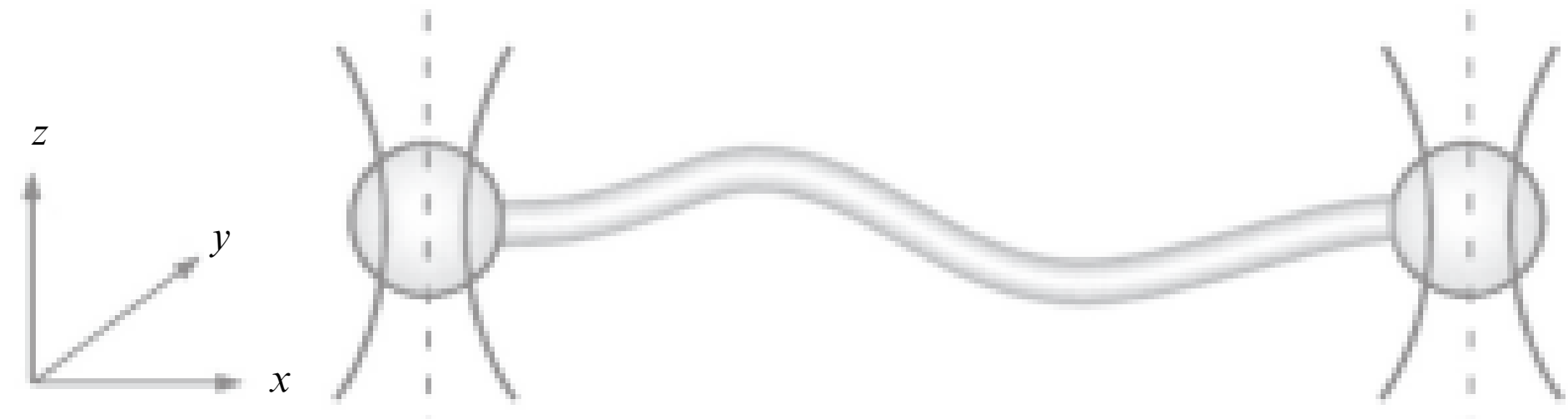
Fig 1: Experimental configuration to observe thermal force fluctuations in a DNA molecule using optical tweezers. Adapted from [1].
